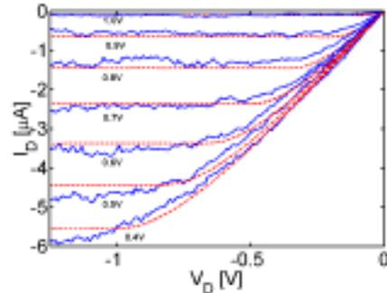
Fig. 7 The experimental  $I_D$  vs.  $V_D$  characteristics of a planar-gated CNTFET (3). The measured characteristics (solid line) are fit by a square law model with series resistance included (the dashed line).
