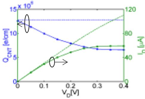
Fig. 4 The charge at the beginning of the channel (on the left axis) and the drain current (on the right axis) vs. the drain voltage at  $V_G=0.4V$  and  $C_{ins}=90pF/cm$  by the charge control model [8] (dashed line) and the new model (solid line). The detailed numerical simulation (circles) shows the charge control model fails at the quantum capacitance limit.
