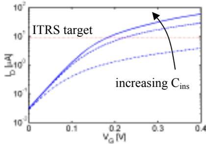
Fig. 5 The drain current vs. the gate voltage for  $C_{ins}=0.4pF/cm$  (the dash-dot line),  $5pF/cm$  (the dashed line), and  $90pF/cm$  (the solid line). The dotted line shows the ITRS target of on-current,  $1500 \mu A / \mu m$ , times  $2d$ , where  $d = 3nm$  is the diameter of the nanotube.
