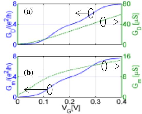
Fig. 6(a) The channel conductance and (b) the transconductance (at  $V_D=0.4V$ ) vs. the gate voltage when  $C_{ins}=0.4 pF/cm$  (shown as the dashed line on the right axis) and  $C_{ins}=90pF/cm$  (shown as the solid line on the left axis).
