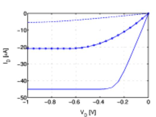
Fig. 8 The theoretical upper limit  $I_D$  vs  $V_D$  of the CNTFET shown in Fig. 7 at  $V_G=0.4V$ . The solid line assumes ideal contacts with zero series resistance and a ballistic channel. The solid line with symbols assumes zero series resistance but includes the channel scattering. The dash-dot line is the measured characteristics.
