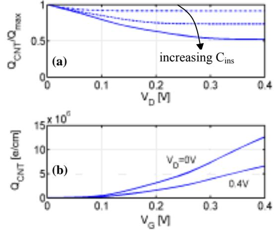
Fig. 3 (a) The normalized electron density at the beginning of the channel vs. the drain voltage at  $V_G=0.4\text{V}$  for three N-type, 3nm-diameter, CNTFETs with  $C_{ins}=0.4\text{pF/cm}$  (dash-dot line),  $5\text{pF/cm}$  (dashed line), and  $90\text{pF/cm}$  (solid line). (b) The charge vs. the gate voltage curves for  $C_{ins}=90\text{pF/cm}$ . The power supply voltage specified by ITRS for the 2016 technology node [15],  $0.4\text{V}$ , is assumed in the subsequent calculations.
