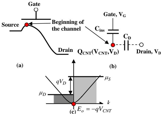
Fig. 2 (a) The subband profile vs. the channel position at a high drain bias and (b) The proposed model of CNTFETs. The gate voltage  $V_G$ , modulates the channel through the gate insulator capacitance  $C_{ins}$ . 2D electrostatics could be included by assuming a drain capacitance,  $C_D$ . (c) At the ballistic limit, the  $+k$  states at the beginning of the channel are filled by the source Fermi level and the  $-k$  by the drain Fermi level.
